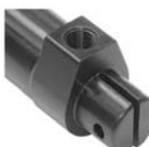
Slotted - .090" slot inline with fitting. 3/16" hole drilled 90° to fitting.
