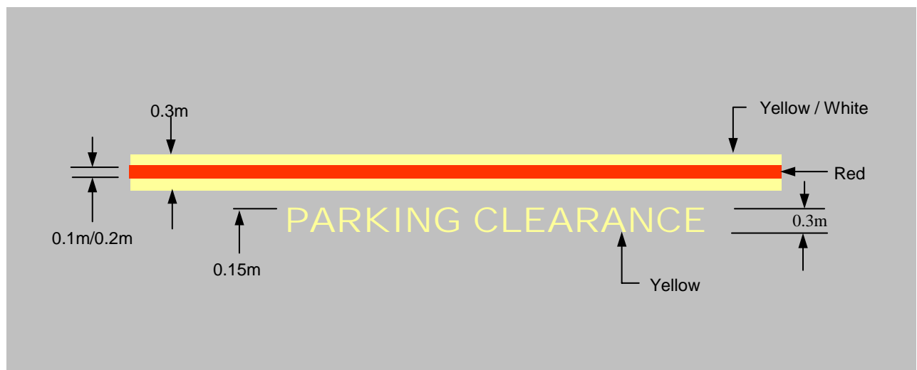
Figure 8.5-1: Parking clearance line
