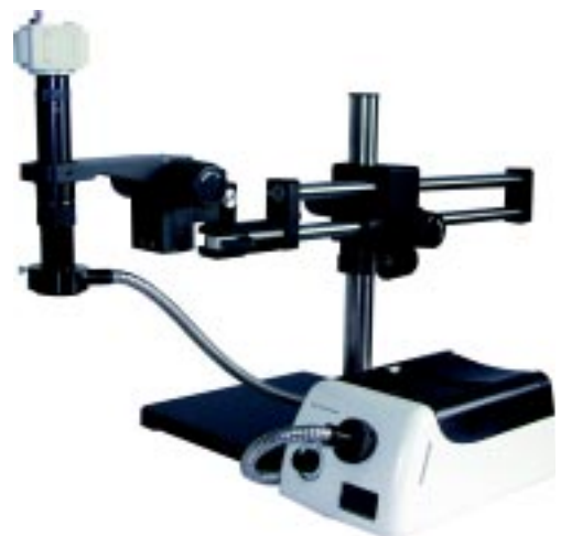
MZ4003 Zoom Lens on Dual Arm Boom Stand with fiber optic illuminator, ring light and GP020101 Color CCD camera
