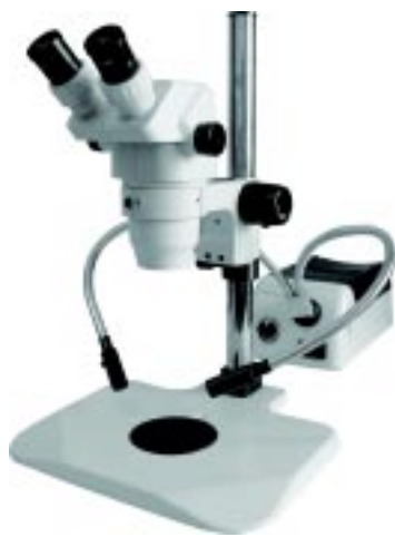
SZ1002 Binocular on Post Stand with Fiber Optic Illuminator and Dual Pipe Light Guide
