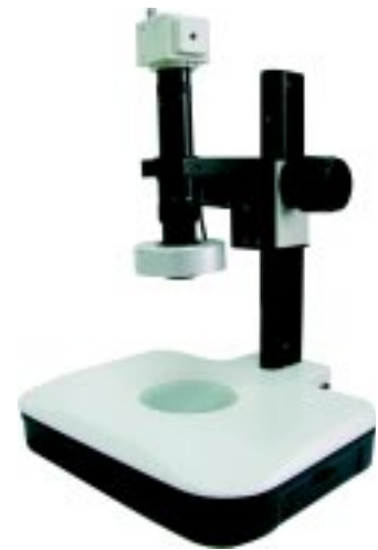
MZ2011 Zoom Lens on Track Stand and MA342101 LED Ring Light
